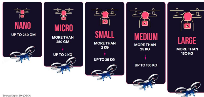
Figure 4. Size-based Classification of Drones (Source: Digitalsky (Directorate General of Civil Aviation, Government of India, n.d.))
